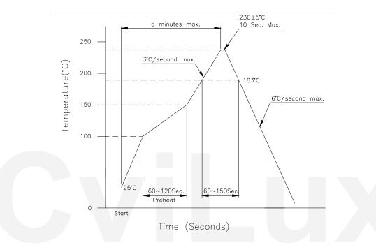
11.2 Using Lead-Free Solder Paste
