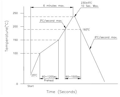
12.2 Using Lead-Free Solder Paste
