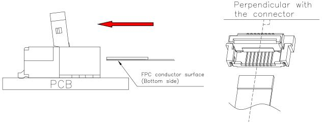
12.1.3 Rotate down the actuator until firmly closed. It is critical that the inserted FFC/FPC is not moved and remains fully inserted.
