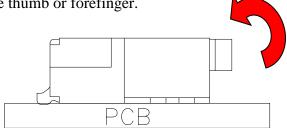
12.1.2 Fully insert the FFC/FPC in the connector parallel to mounting surface, with the exposed conductive traces facing down. And ensure that the FFC/FPC is properly inserted into the connector insertion slot.
